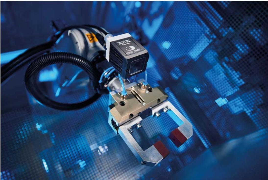
*Fig. 1: The VISOR® Robotic sensor supplies the robot with all image data in robot coordinates. Common 2D robotics applications can be easily and conveniently set up in the configuration software.*
