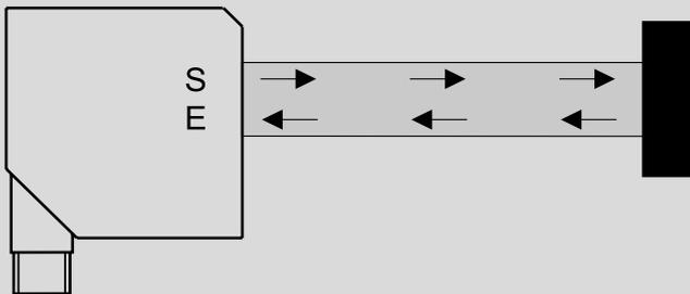
The transmitter and receiver of a diffuse sensor are accommodated in a single housing. The light emitted by the transmitter hits the target object, which reflects the light. This returning light is evaluated by the receiver. The advantage of this method is that no reflector is required.
