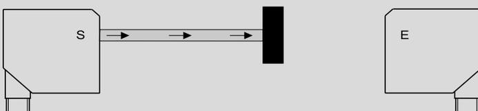
A photoelectric through-beam sensor has a separate transmitter and receiver. This means that light only travels the path between the transmitter and the receiver once. For this reason one speaks of photoelectric through-beam sensors.
