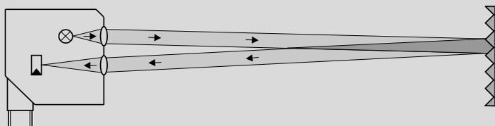
The transmitter and receiver are accommodated in a single housing in photoelectric retro-reflective sensors. The light emitted by the transmitter hits a reflector and is reflected. The receiver evaluates the reflected light. The advantage lies in the small size of the reflector. It is also easy to install because it is a passive element and thus requires no connections.
