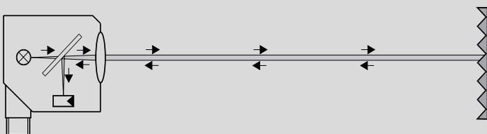
With photoelectric retro-reflective sensors one speaks of the autocollimation principle when the light reflected from the reflector travels parallel to itself (i.e. within itself). The light emitted by the sensor hits a reflector and is reflected. The reflected light is then deflected to a receiver by a semi-transparent mirror and evaluated.
