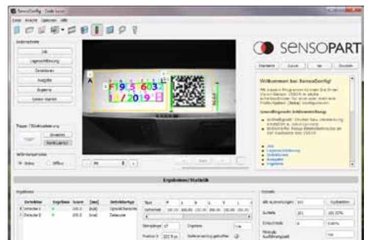
Fig. 4a+b: The VISOR® V20 code reader from SensoPart reads both DMC and clear text and can also export quality parameters. All elements are recorded and analysed in a reading process.
