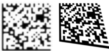
Fig. 3: Typical code errors (e.g. too faint or distorted) can be detected using standardised quality parameters so that the source of error can be eliminated. The VISOR® code reader from SensoPart offers the option of exporting the quality parameters for each code that has been read, so that hard-to-read codes are immediately detected.
