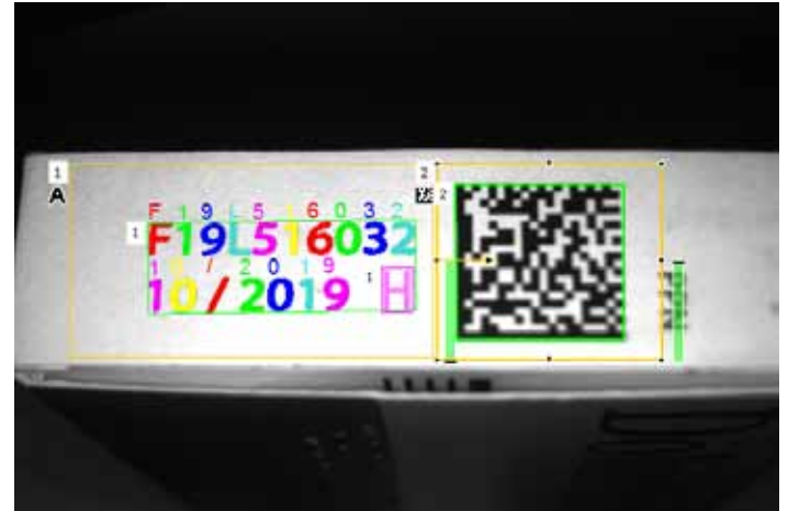
Fig. 2: Each pharmaceutical packaging is rendered unique by the application of a unique identifier during production. Good readability is essential for later code checks.
