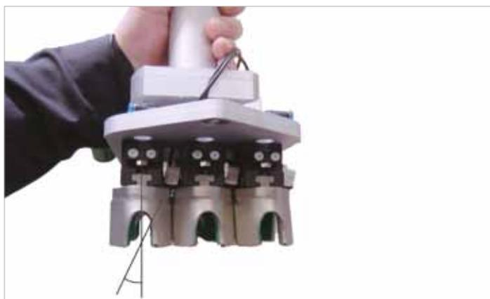
Fig. 3: The sensors are positioned at an angle of approx. 60° and a scanning distance of 20-25 mm.
