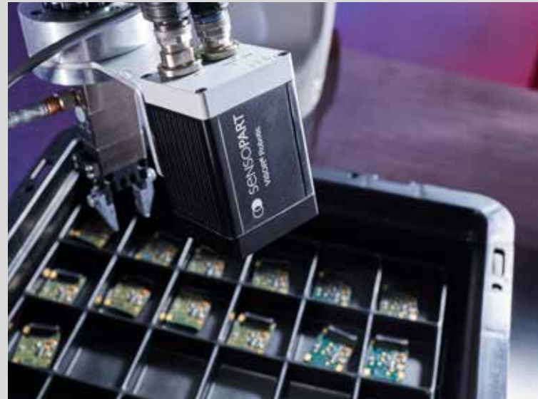
The VISOR® Robotic detects the component's position in a universal tray. It can then be reliably removed. Up to 255 configurations enable utmost production flexibility.
