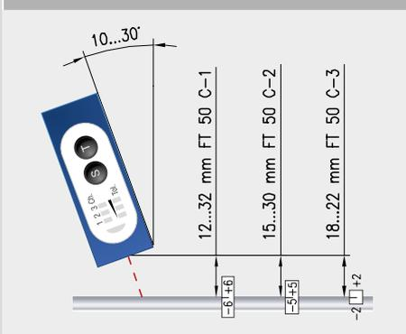
The depth of field of the FT 50 C also varies depending on the light spot geometry:
