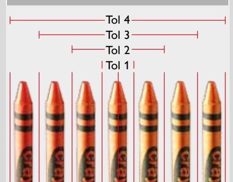
The detection window can be adapted by adjusting colour selectivity.
