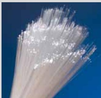
Fibre-optic cables differ in the transmission material used – glass or plastic. SensoPart offers the so-called fibre material in both variants. Glass fibres are highly resistant to chemicals and high temperatures. Suitable metal or silicone sheath materials allow the use of glass fibres in harsh environmental and process conditions. Larger glass-fibre cross-sections offer high functional reserves and reliability, even in dusty and dirty environments.
